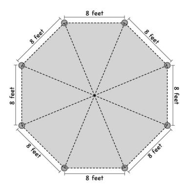
The perpendicular distance from any one "wall" to the center of the Ramada is 9.7 feet.
